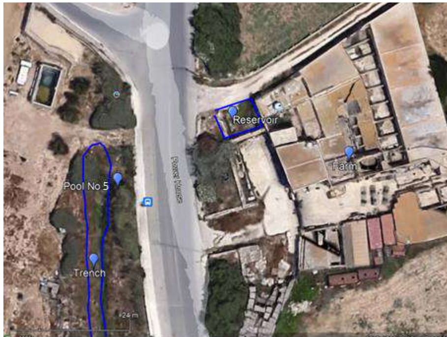
FIGURE 16: GOOGLE IMAGE SHOWING THE RESERVOIR (SUMP OR PIT) COLLECTING RUNOFF FROM THE CATCHMENT AND DIRECTED TO THE TRENCH ON OPPOSITE SIDE OF THE ROAD
