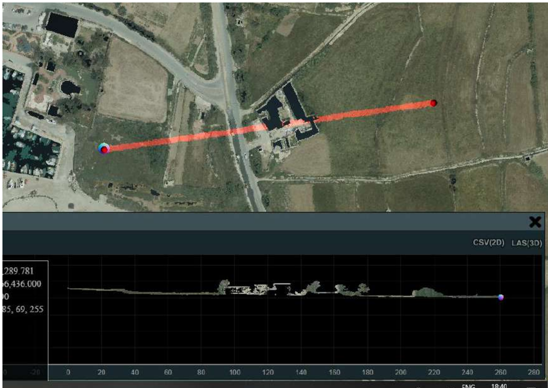
FIGURE 104: CROSS-SECTION ACROSS THE AQUIFER FROM THE EAST (LEFT) TO THE COASTLINE ON THE RIGHT (WEST) DERIVED FROM LIDAR DATA
